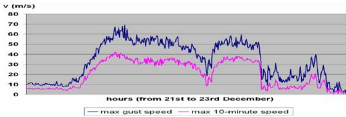
Figure 2 Maximum recorded wind speed: Maslenica bridge 22nd December 1998: 69,0\text{ m/s} = 248.4\text{ km/h}
