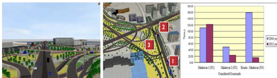
Figure 7 View on the three-level flyover model fragments in 3D Animation (on the left) and the average delay time in the problem zones for 2004 and 2012 (on the right)
