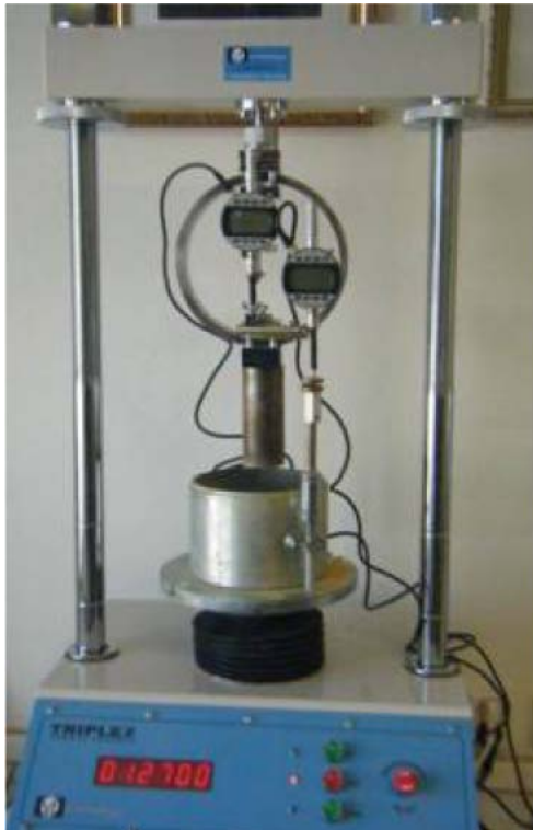
Figure 6 Apparatus for determining M_{R,CBR} (laboratory of Mendel University in Brno)
