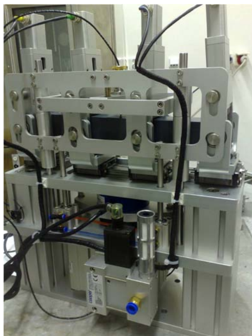
Figure 2 Device for measuring the stiffness of the modules 4-point test according to EN 12697-26
