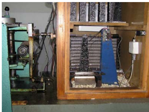
Figure 1 The device for measuring modulus stiffness 2-point test according to EN 12697-26
