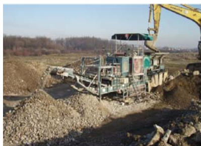
Figure 3 Sopnica-Jelkovec Site: Recycling of Material on Site (a) and Recycled Material (b)
