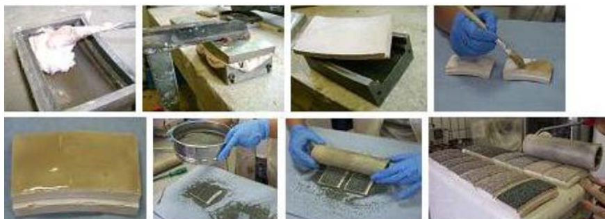
Figure 2 Preparation of sand specimens for the accelerated polishing wheel.
