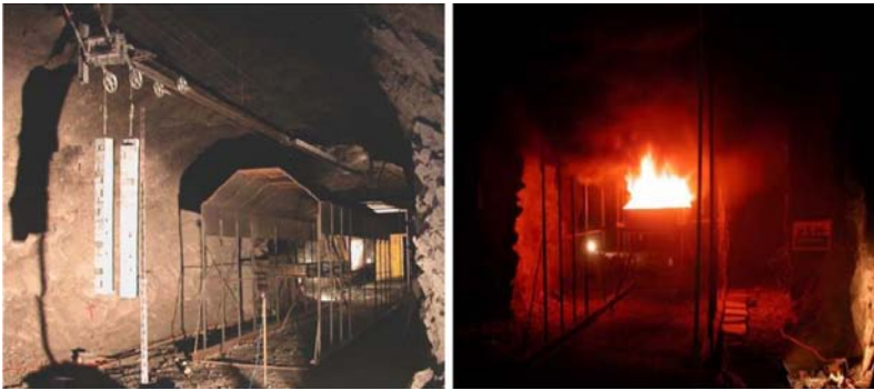
Figure 7 Fire testing of KT in a tunnel.
