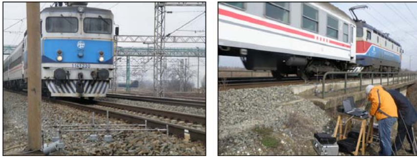
Figure 7 Deflection measurement (left: track in embankment, km 0+371; right: track on the bridge, km 5+398)
