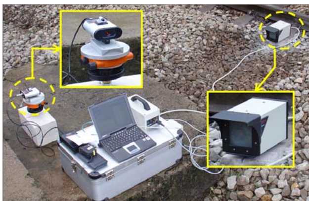
Figure 6 Measuring equipment mounted on the railway track
