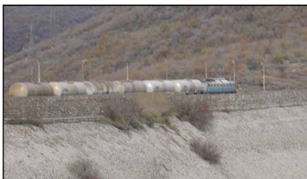
Figure 8 Freight train (second live load)
