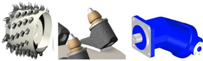
Figure 4 The main elements of milling heads systems
