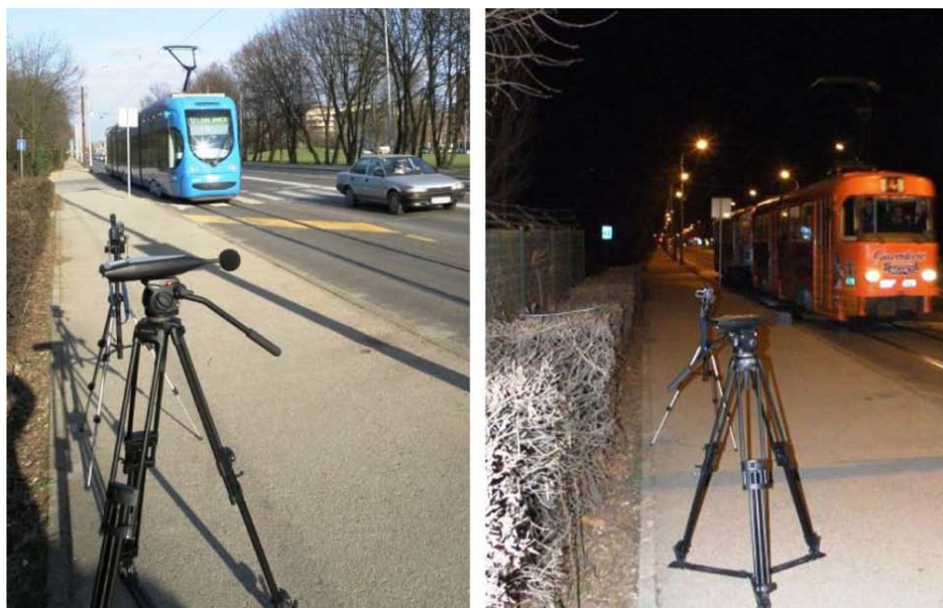
Figure 3 Measuring noise levels and recording of the traffic load at MP2
