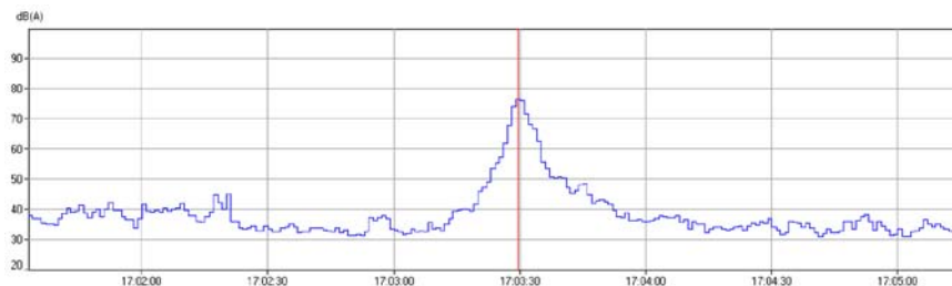
Figure 1 Equivalent noise levels during the tilting train passage.
