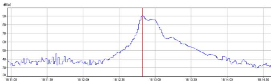
Figure 2 Equivalent noise levels during the cargo train passage.
