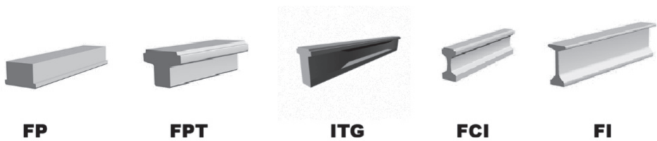
Figure 1 The different types of bridge beams [10], where FP: Ferrobeton (Manufacturer) Pontterv (Designer); FPT: Ferrobeton (Manufacturer) Pontterv (Designer) T (cross section); ITG: I (cross section) Támasztó (Support) Gerenda (Beam); FCI: Ferrobeton (Manufacturer) Composit I (Cross section); FI: Ferrobeton I (Cross section)
