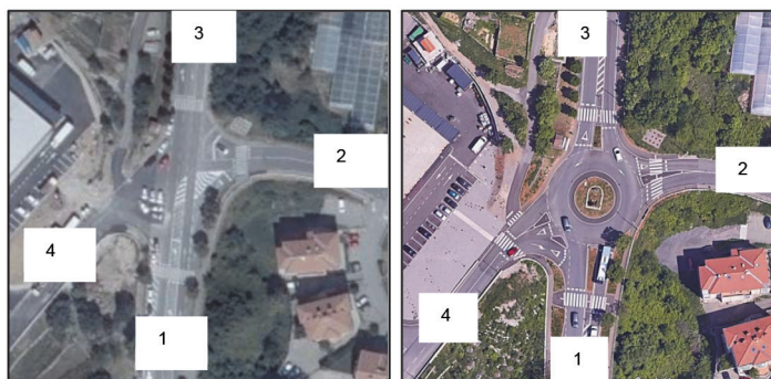
Figure 1 Analyzed intersection: conventional unsignalized intersection – before reconstruction (left) and roundabout – after reconstruction (right)
