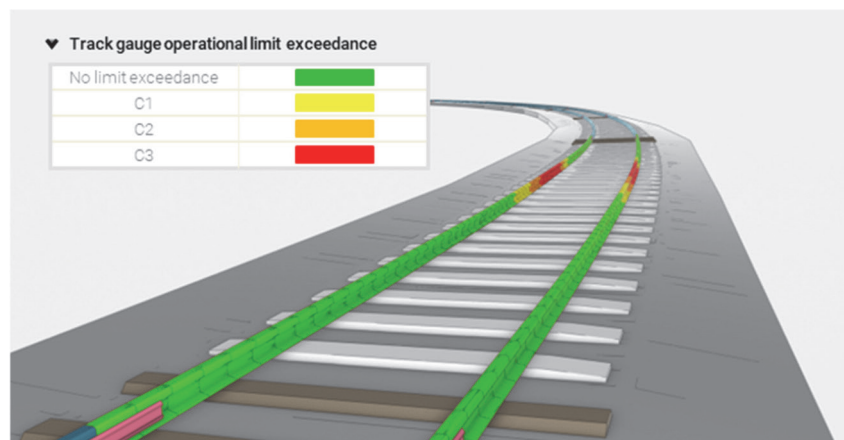
Figure 4 BIM-based track model visualization illustrating track gauge compliance
