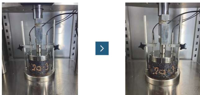
Figure 2 Laboratory device for static (left) and dynamic (right) testing of asphalt mixture creep
