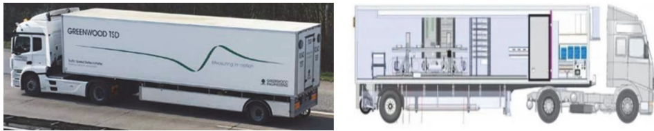
Figure 2 Traffic Speed Deflectometer (left); Schematic (right) [18, 19]
