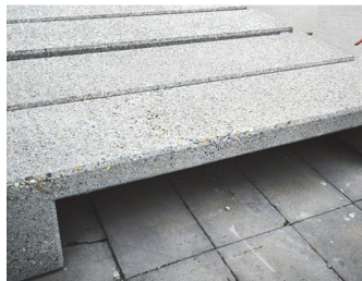
Figure 3 Poured concrete bench (CB) with WBA as partial aggregate replacement
