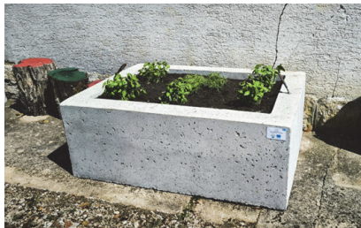
Figure 2 Concrete planters (CP) with WBA as partial aggregate replacement
