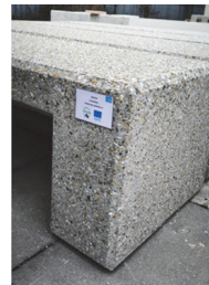
Figure 3 Poured concrete bench (CB) with WBA as partial aggregate replacement
