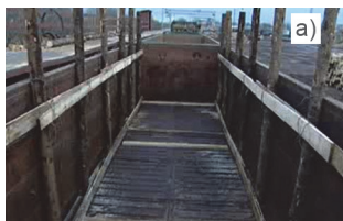
Figure 3 A placement of wooden posts in an open wagon body: a) an inside view, b) a side view
