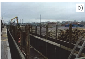
Figure 3 A placement of wooden posts in an open wagon body: a) an inside view, b) a side view
