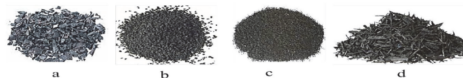
Figure 1 Different sorts of rubber aggregates: a) chipped, b) crumb, c) granular, d) fibre (Zrar and Younis) [1]
