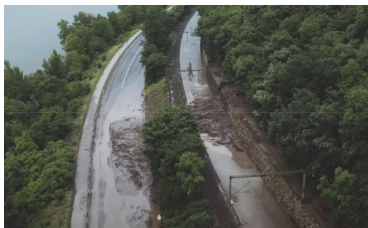
Figure 1 The landslide that covered the railway tracks and main road in the Danube Bend in 2022 [9]
