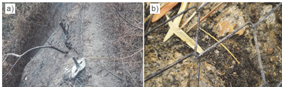
Figure 6 a) detail of the upper part of the membrane after the fire passed, b) wire surface condition in some areas of the mesh after the fire
