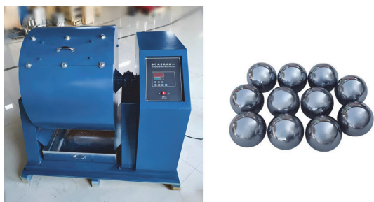
Figure 2 Los Angeles abrasion testing apparatus with steel charging balls [5]
