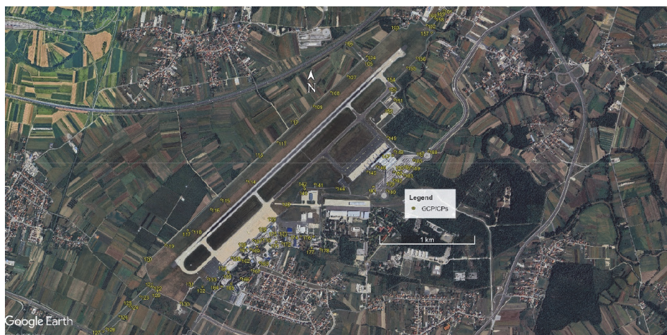
Figure 1 Distribution of Ground Control Points (GCPs) and Check Points (CPs) across the airport area
