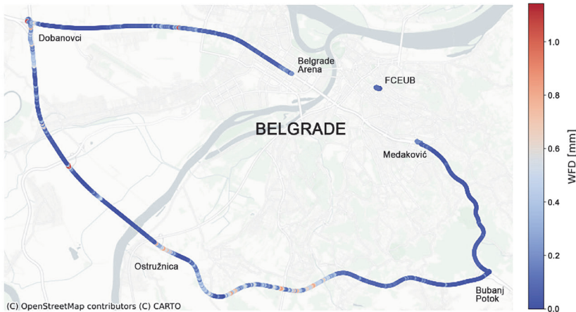
Figure 3 Spatial distribution of measured WFDs along selected motorway sections near Belgrade
