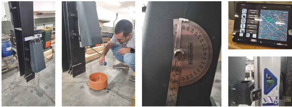
Figure 4 Laboratory tests of MARWIS sensor accuracy for WFDs measurements
