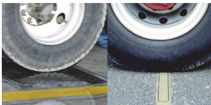
Figure 3 Wheels over a plate and a strip WIM sensor
