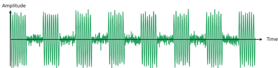
Figure 9 Sound wave profile representation for forced flow traffic
