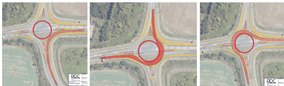
Figure 8 Vehicle tracking analysis for the temporary roundabout, phase 2 tracking 1, 2 and 3 [2]
