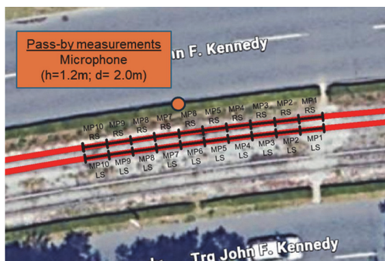
Figure 3 Measurement setup for rail roughness and pass-by noise measurements
