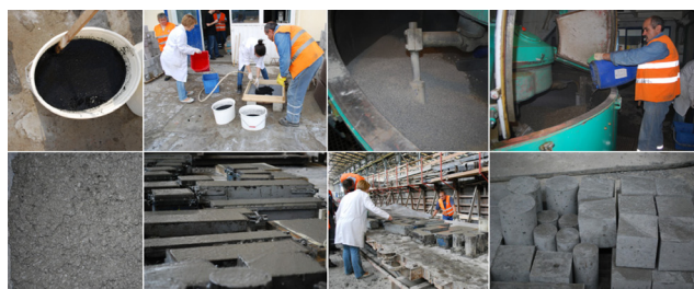
Figure 2 Preparing the samples in the precast concrete plant TBP Pojatno, Viadukt d.d. [2]
