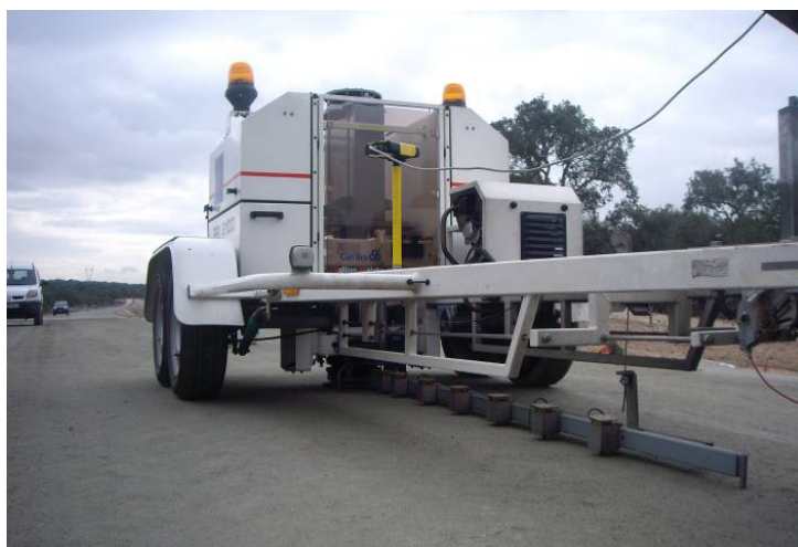
Figure 1 Falling Weight Deflectometer equipment.
