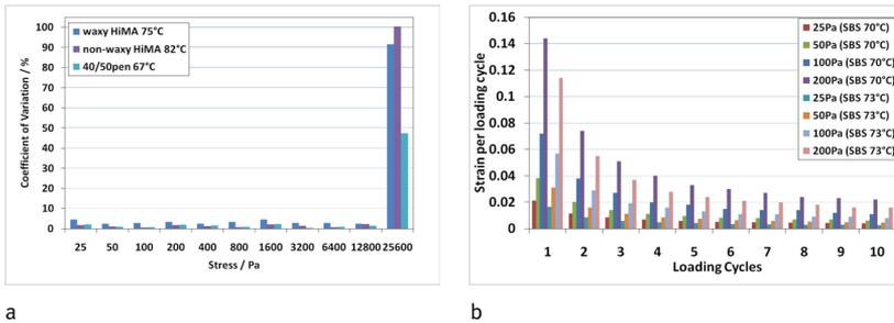
**Figure 3** (a) Coefficient of variation of the strain values for the 10 loading cycles applied at each stress level for the different binders at their SHRP ( $G^*/\sin\delta = 1\text{ kPa}$ ) rutting test temperature. (b) Strain values for 10 loading cycles applied at stress levels of 25, 50, 100 and 200Pa for the SBS 70°C and SBS 73°C.
