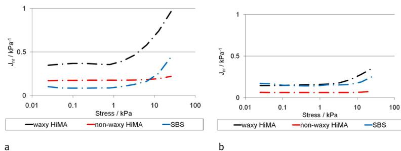
**Figure 6** (a) Non-recoverable compliance at different stress levels of bituminous binders at 55°C. (b) Non-recoverable compliance at different stress levels of bituminous binders after RTFOT-aging at 55°C.
