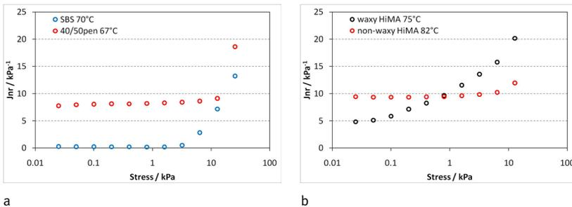
**Figure 1** Comparison of  $J_{nr}$  values at various stresses of (a) an unmodified binder (40/50 open) and a modified binder (SBS-modified), (b) a waxy and a non-waxy HiMA binder at their SHRP ( $G^*/\sin\delta = 1\text{ kPa}$ ) rutting test temperature.
