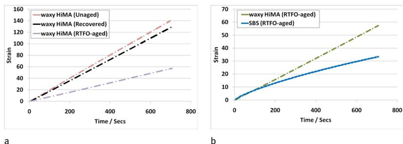
**Figure 7** (a) Strain deformation curves for the unaged, RTFO-aged and recovered waxy HiMA binders at 55°C for 1000 loading cycles at a 0.1 second creep load followed by a 0.6 second rest period at a stress of 3200Pa. (b) Strain deformation curves for the RTFO-aged waxy HiMA and SBS-modified binders at 55°C for 1000 loading cycles at a 0.1 second creep load followed by a 0.6 second rest period at a stress of 3200Pa.
