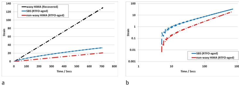
**Figure 8** (a) Strain deformation curves for the binders at 55°C for 1000 loading cycles at a 0.1 second creep load followed by a 0.6 second rest period at a stress of 3200Pa. (b) Log-log plot strain deformation curves for the SBS modified binder and the non-waxy HiMA at 55°C for 1000 loading cycles at a 0.1 second creep load followed by a 0.6 second rest period at a stress of 3200Pa.
