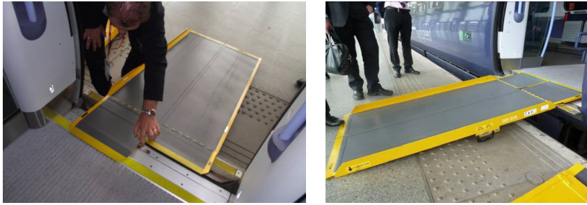
Figure 2 Manual mobile Ramp (Port-a-Ramp, UK), bridging the gap between the train and the platform (South Eastern Trains, England)
