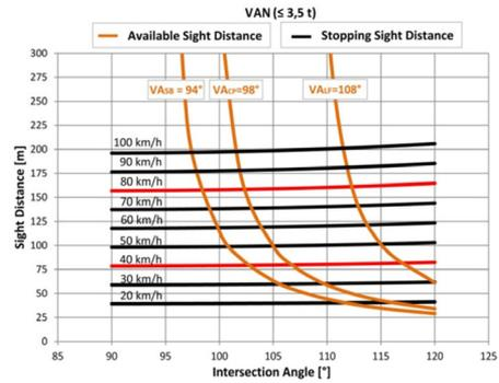
Figure 3 Sight distance nomographs for passenger car and van ( $\leq 3,5$  t)
