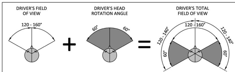
Figure 5 Figure 5. Driver's total field of view
