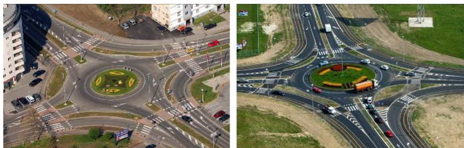
Figure 6 Single-lane roundabout with additional lanes for the right turn
