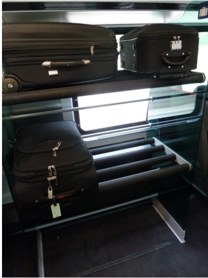
Figure 7 Wrong dimensions of luggage racks lead to inefficient storage
