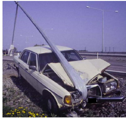
b) Deformable column [4]
