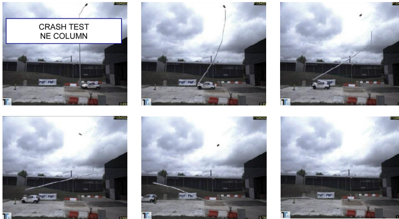
Figure 5 Crash test with a non-energy absorbing column [7]
