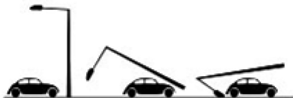
Figure 4 Non-energy absorbing column behaviour [6]
