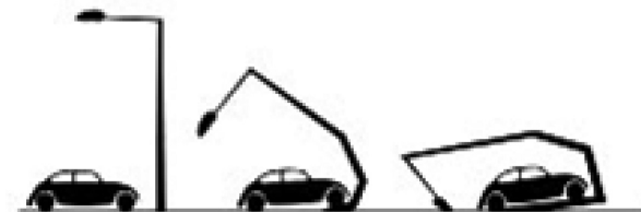
Figure 7 High energy absorbing column behaviour [6]
