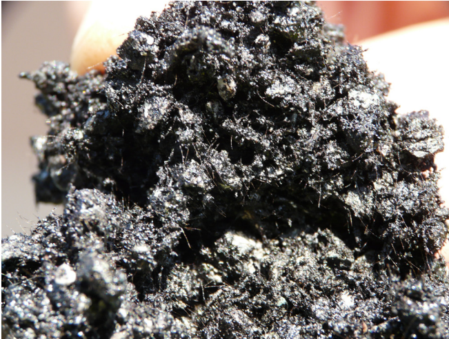
Figure 1 Fibers used in GRIPFIBRE® mix design
