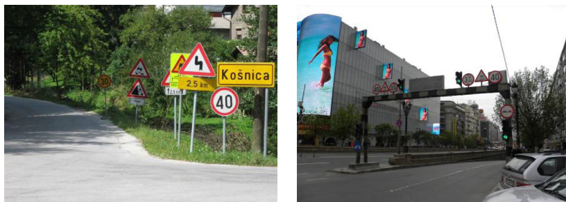
Figure 8 The Road user cannot read the information (too much information at once and/or distraction)
