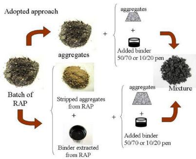
Figure 2 Adopted procedure for simulating a perfect blend of the virgin added binder and the binder in the RAP
