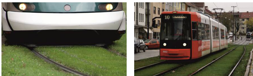
Figure 4 Illustration of the extremely limited space between the vegetation and the underbody of Strasbourg's Eurotram (left). In Bremen the more distinctive vertical spacing between top of rail and vegetation is clearly visible and resembles low vegetation (right)
