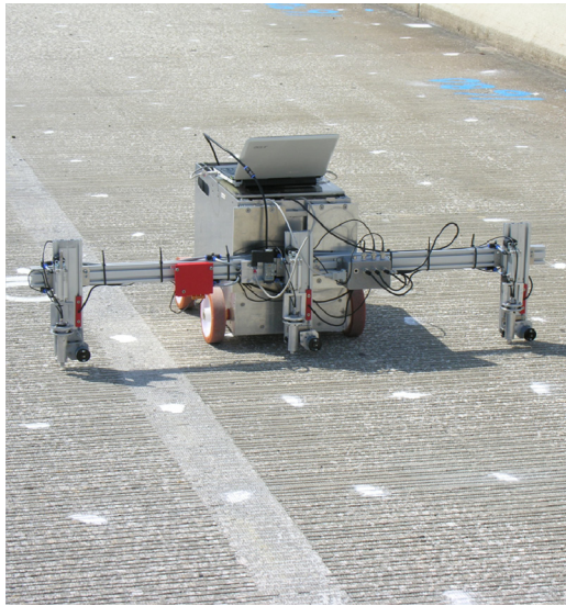
Figure 3 Delamination detection using IE (left) and GPR survey (right).
