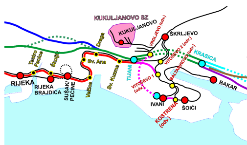
Figure 3 New railway connection at Vitoševo (direct link between Ivani and Rijeka and Brajdica) – (stage III of the junction construction)
