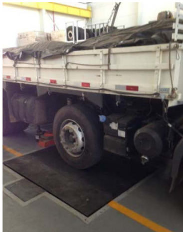
Figure 4 Weighing scale used for the calibration and example of the spring calibration
