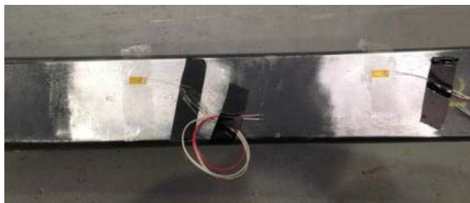
Figure 3 Primary suspension spring leaf instrumentation
