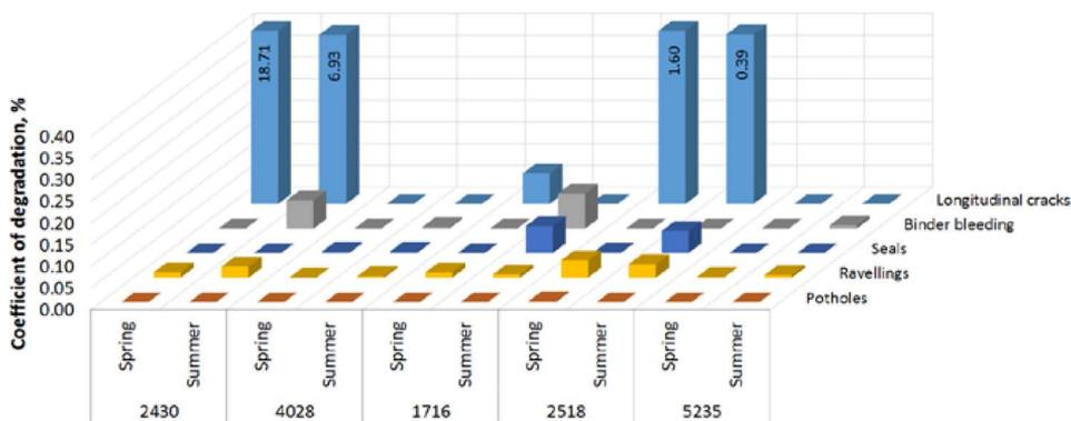
Figure 4 Results of the visual assessment of the trial sections with soft asphalt
