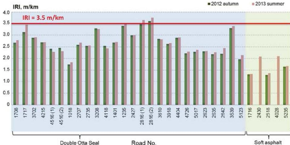
Figure 3 Roughness of trial sections with double Otta seal
