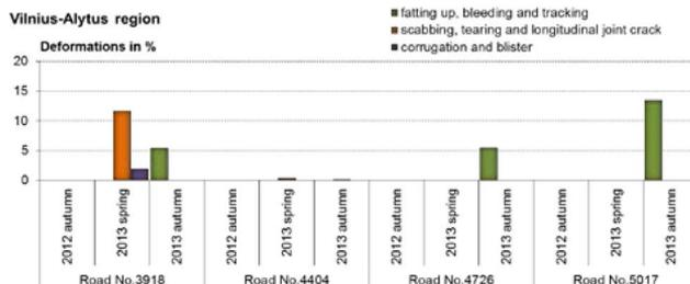
Figure 5 Results of the visual assessment of the trial sections with double Otta seal
