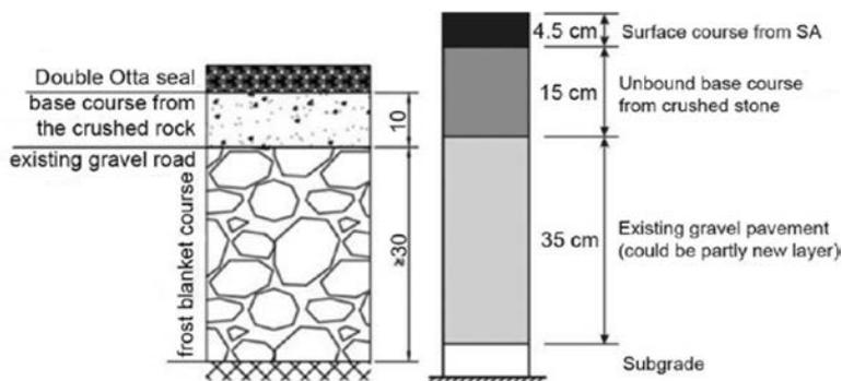
Figure 1 The structure of double Otta seal (on the left) and soft asphalt pavement (on the right)
