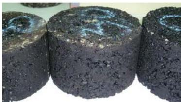
Figure 2 Laboratory asphalt specimens
