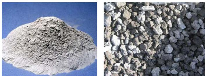
**Figure 1** Industrial waste materials: fly ash (left) and slag (right)
