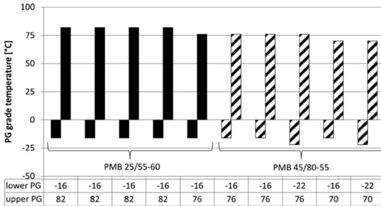
Figure 1 Performance gradation of tested polymer modified bitumen
