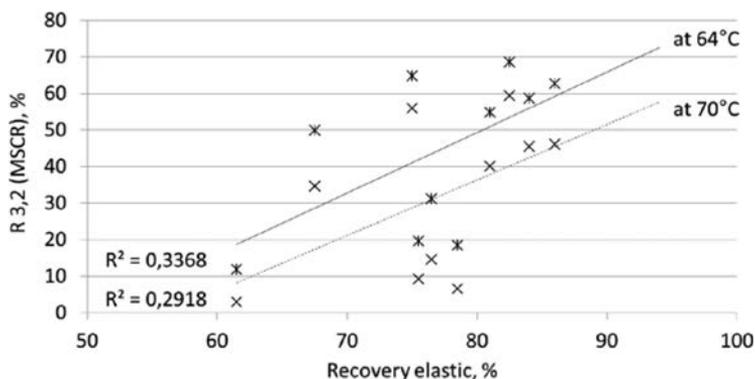
Figure 4 Relationship between elastic recovery from ductility and elastic recovery from MSCR
