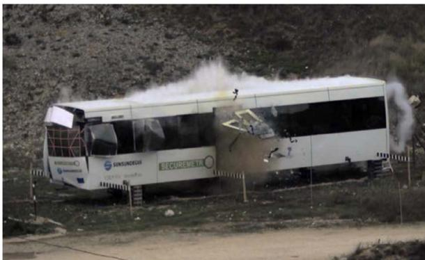
Figure 3 High-speed image of the trial with the demonstrator carriage
