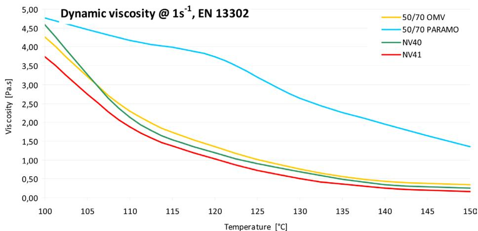
**Figure 1** Dynamic viscosity (viscosity curves) at shear rate of 1 s<sup>-1</sup> and temperature interval 100-150°C
