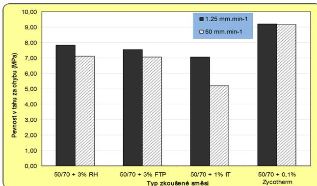
Figure 3 Results of flexural strength test, set II
